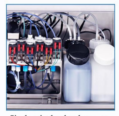
Single print head and recovery diaphragm pump design makes more stable and durable.
